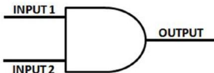
**Figure 6-4.** The AND Logic Gate circuit symbol
