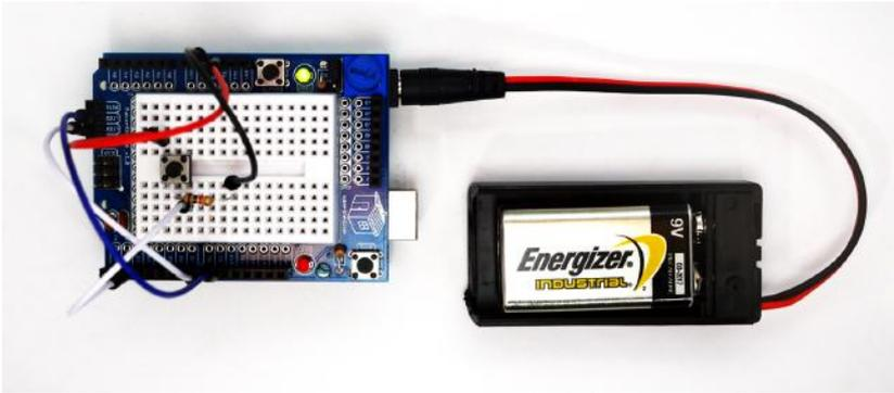
**Figure 5-1.** *The Arduino NOT Logic Gate*
